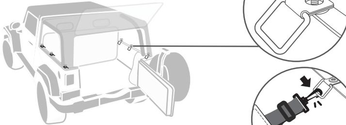
**Step 2** Snap the clips onto the rings with the cover logo side up.
